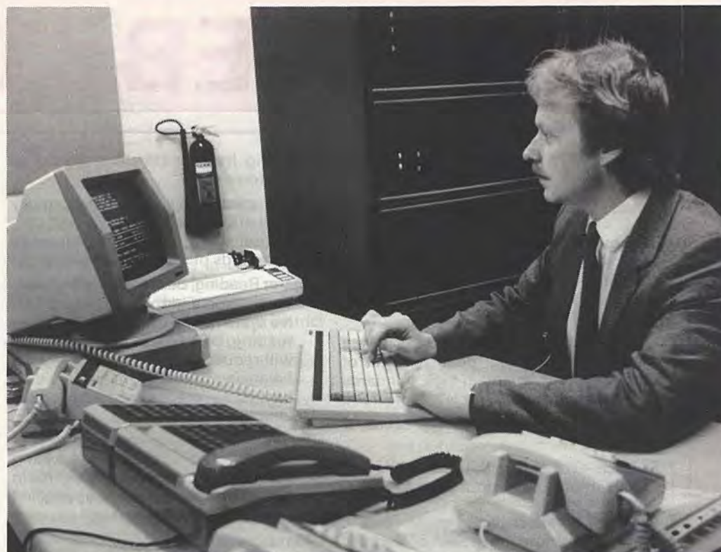
Author Tony Timmins checks the telephone system at North Wirral, using the computerised maintenance equipment, which can programme changes in the system
