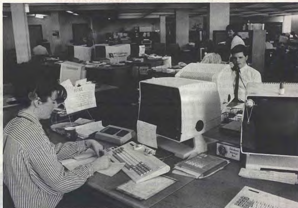
The automatic call distribution system in operation in North Wirral, where accounts queries come direct to operators at V.D.U.s with direct access to customer accounts records. Rachael O'Connell and David Higgett can be seen at two of the terminals
